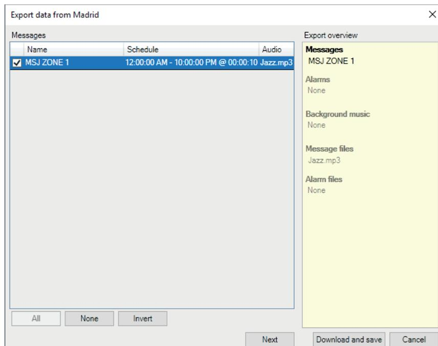
Select the scheduled messages you want to load to the destination device. The files necessary for playback will be loaded automatically.
