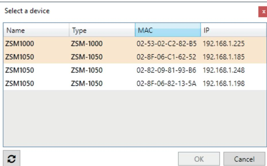
Once the configuration parameters have been entered, click on the Devices menu option, and the window with access to all the configured devices will appear. Double-click (or right-click ->Connect) to connect to the device. If you added access to one or more groups, you can access them in the Groups option of the menu.
