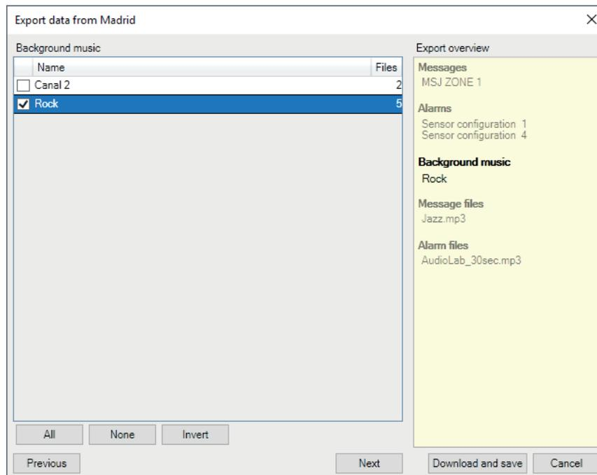
Select the alarm files you want to upload to the target device. If you have previously selected alarms that have associated audio files, these files will be marked as obligatory.
