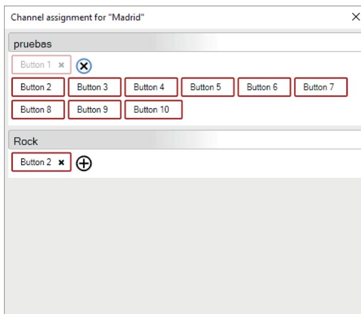
To set, press the "+" icon. This will scroll through the available buttons. To remove the setting, click on the "X" icon on the button label.
