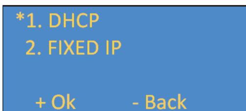
Allows you to configure the device with DHCP or FIXED IP.
