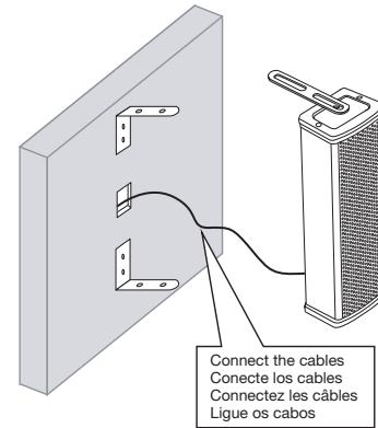
**NOTE:** keep the wiring isolated to avoid accidents or unwanted manipulation (e.g. in an ABS box).
